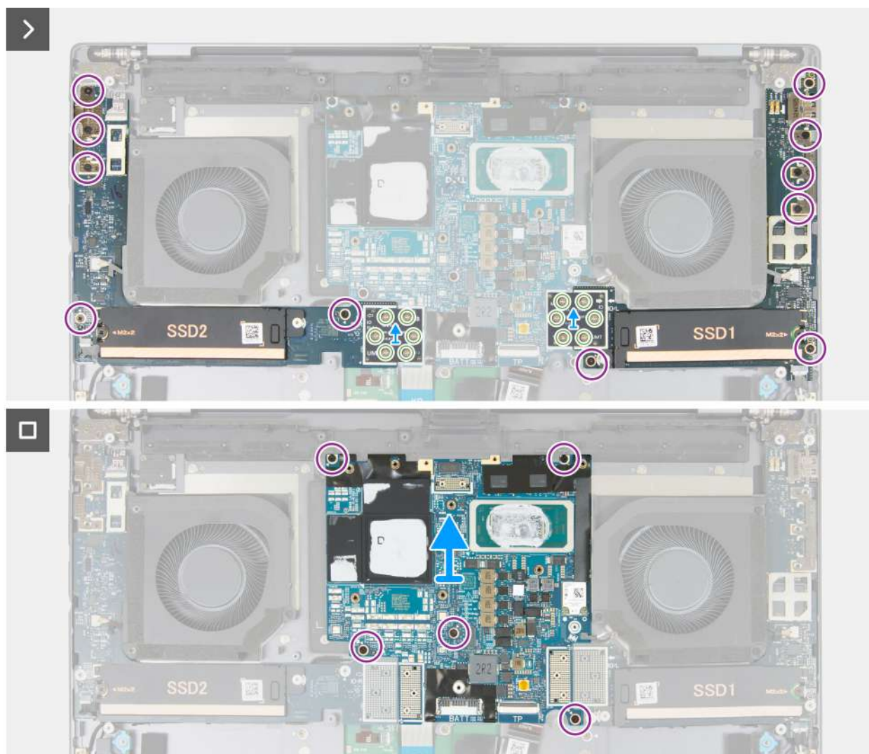
Figure 56. Removing the system board (integrated graphics)
