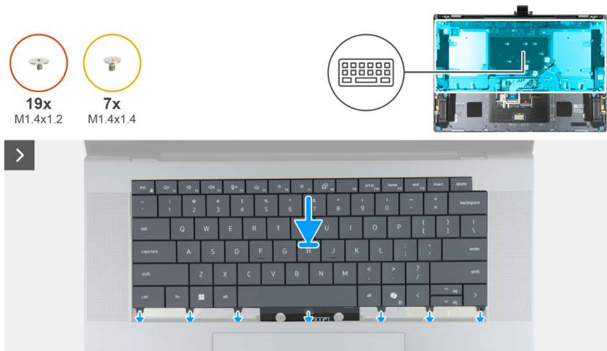
Figure 79. Installing the keyboard
