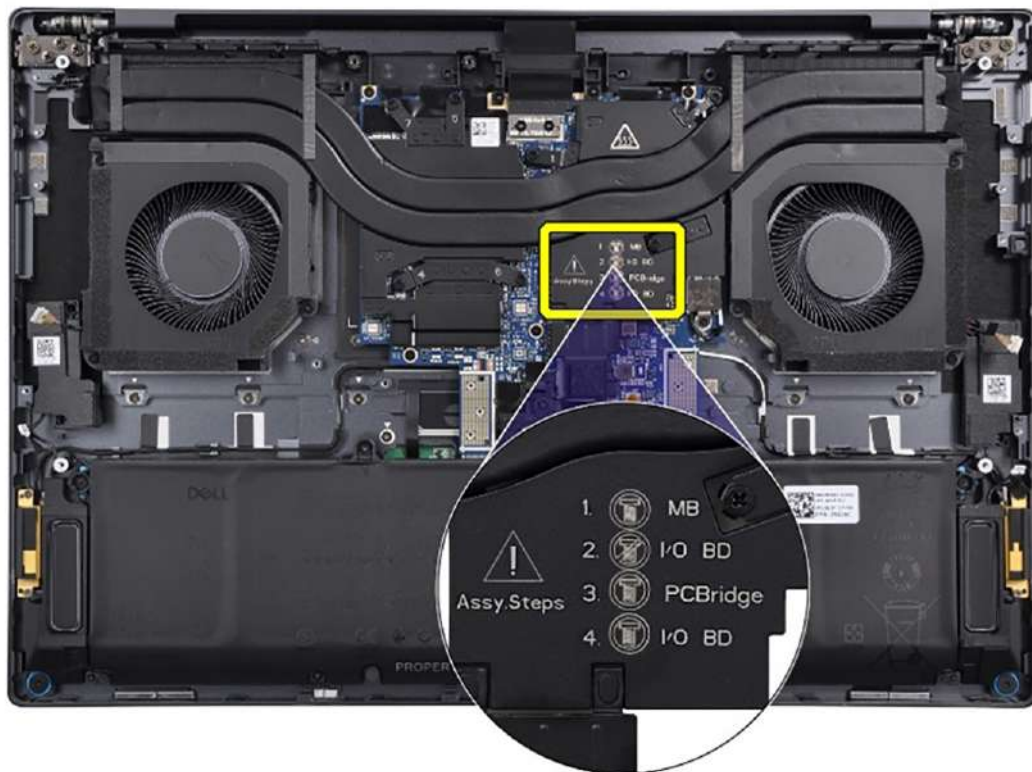
Figure 66. Assembly steps printed on heat sink
