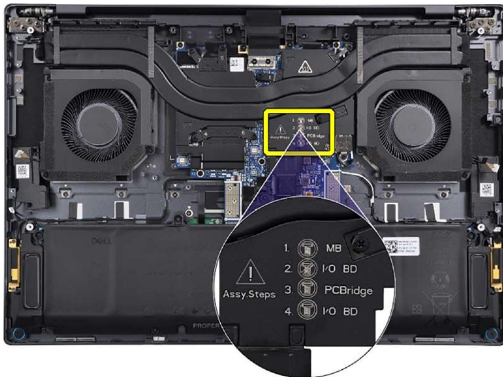
Figure 62. Assembly steps printed on heat sink
