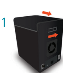
1 While holding the clip in the back, slide back the top cap.
